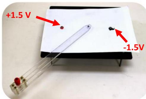
U-type probe on a carbon-coated conductive plate
