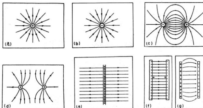
Fig. 1. Lines of electric fields created by different charge distribution: (a) positive charge (b) negative charge (c) a pair of positive and negative charges (d) two positive charges (e) an infinite plate with positive charge (f) two parallel infinite plates with opposite charge (g) two parallel finite plates with opposite charge
