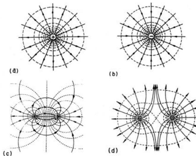
Fig. 2. Equipotential lines (dotted lines) and electric field lines (solid lines) under different charge distributions. (a) positive charge (b) negative charge (c) positive-negative charge pair (d) two positive charges
