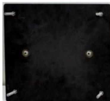
Carbon-coated conductive plates with point-point electrodes
